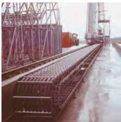
35 chains with supporting frame applied to De Icing equipment at München airport (Germany). The length of the travel distance is 90 m and it's velocity is 90 m per minute.
